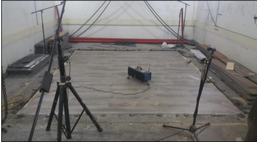
Photo No. 1 Source Room View of Test Specimen Installation
